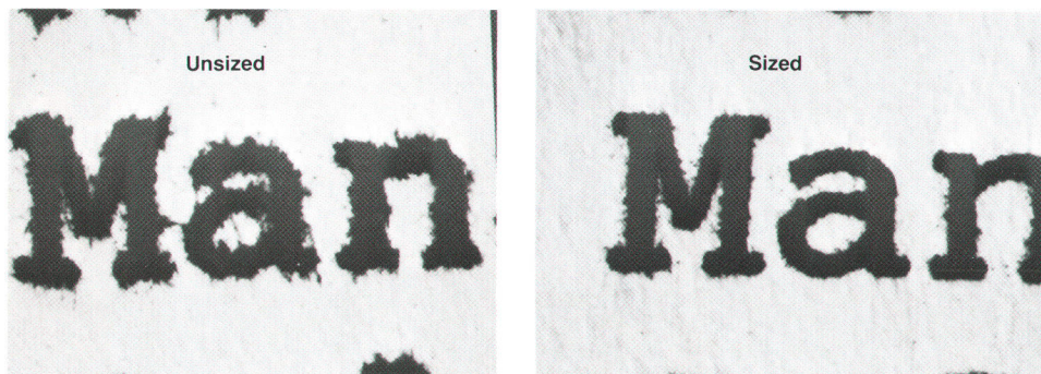
Fig. 6. Photographs of print made on a standard office copier paper before and after starch addition at the size press.
